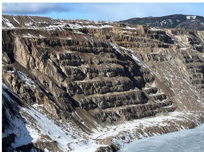
Figure 14.10 View of Pit Wall Showing Difference Between Skree and Rock Profiles Source: AMPL, 2025
